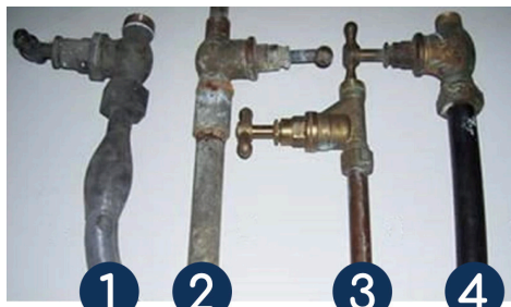
1. Lead 2. Galvanized Steel (Iron) 3. Copper 4. Plastic (Black/Blue Color)
